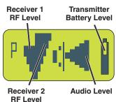
Main Window shown here is used during operation to display RF and audio levels, transmitter battery status, pilot tone status and diversity activity for both receivers.
