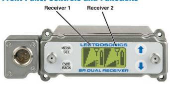
The control panel is a rugged, dust and water resistant design with membrane switches for the control interface. A backlit, graphicstype LCD is used to set up and monitor the receiver. Navigation through the menus is straightforward with text prompts for value and mode selections. The
