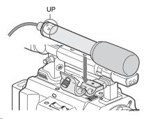
3 Close the microphone holder cover for the original condition to secure, then connect the microphone cable to the AUDIO IN connectors (CH-1 and CH-2) and secure the cable at the cable clamp under the holder.
