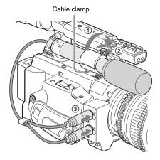
Connect the white plug of the supplied microphone to the CH-1 connector of the camcorder and the red plug to the CH-2 connector.
