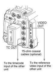
The timecode to be output from the TC OUT connector depends on the setting of "TC Out" on the TC/UB SET menu. If "TC Out" is set to "Generator," the timecode generated by the timecode generator of the camcorder is output during recording and playback. If "TC Out" is set to "Auto," the timecode generated by the timecode generator is output during recording, and that superimposed with the video signal is output during playback.
