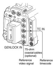
Thus the built-in timecode generator of your camcorder locks to the reference timecode. The message "EXT-LK" is displayed on the screen.
